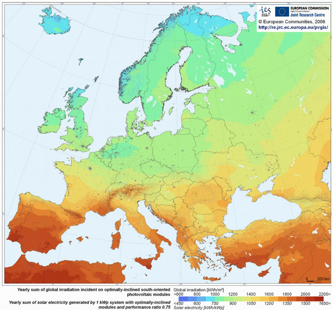
**Figure 12: Extent of global irradiation and photovoltaic solar energy potential in Europe**
